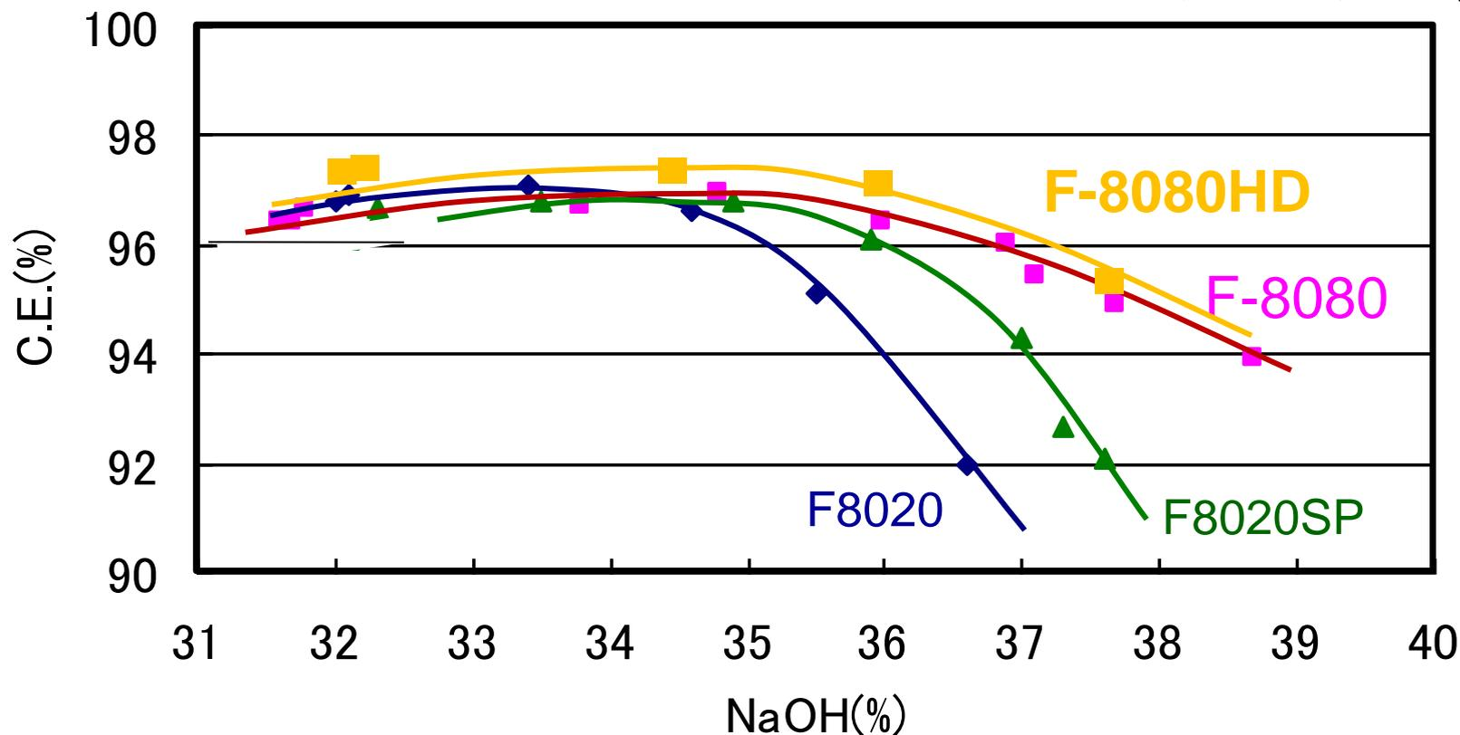
**F-8080 series keep good current efficiency over widest range of NaOH strength**
