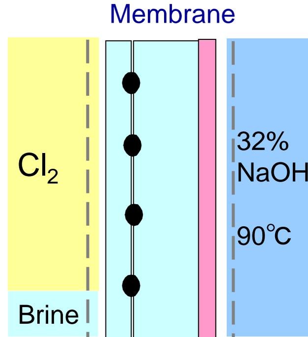
Cl<sub>2</sub> gas stagnation on anode side and high caustic strength on cathode side. In this condition, membrane will have salt crystals.
