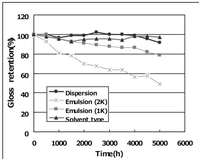
**Figure 4. Accelerated weathering test result (QUV)**
