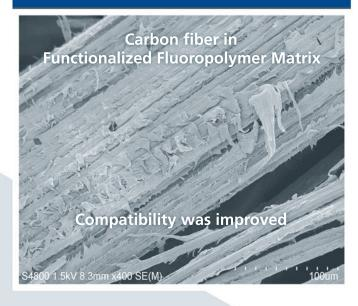
**Surface modification of CFRTP**
