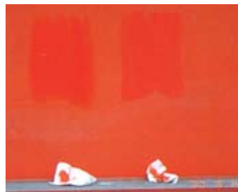
Alkyd coating: chalking and color fade have occurred
