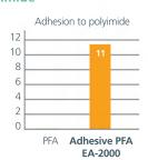
Fluon+ EA-2000 provides better adhesion to PI and Cu as compared to neat PFA without sacrificing original performance.
