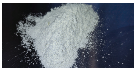
1.32 g of jojoba oil absorbed in 1 g of RESIFA SOLESPHERE H-33 silica is dry, but a bit clumpy
