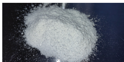
0.5 g of jojoba oil absorbed in 1 g of RESIFA SOLESPHERE H-33 silica is still a fine powder
