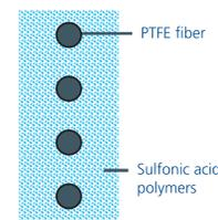
Versatile fluorine-based ion exchange membrane with a wide range of ion exchange capacities
