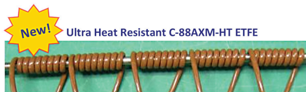
Fig. 2 — Stress crack improvement of Fluon C-88AXMP-HT versus standard ETFE pre-aged three hours at 225°C before coiling and six hours at 225°C after coiling.
